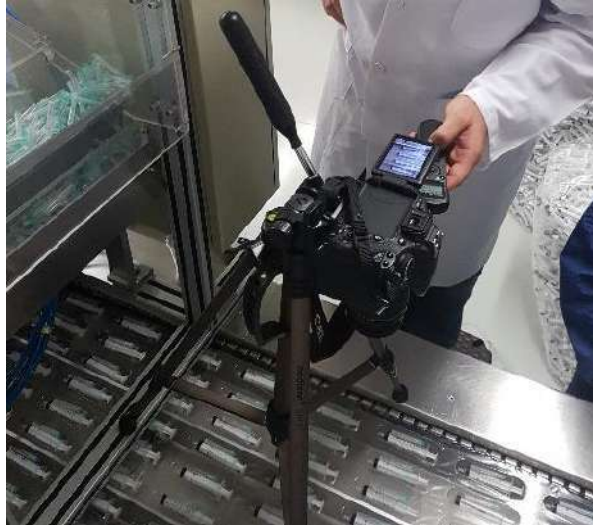
Figure 2. The mechanism established to capture the image in the packing line
