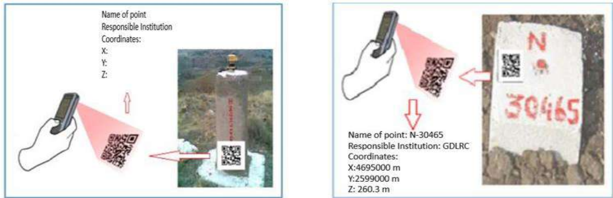
Figure 5: QR code application for ground control points.
