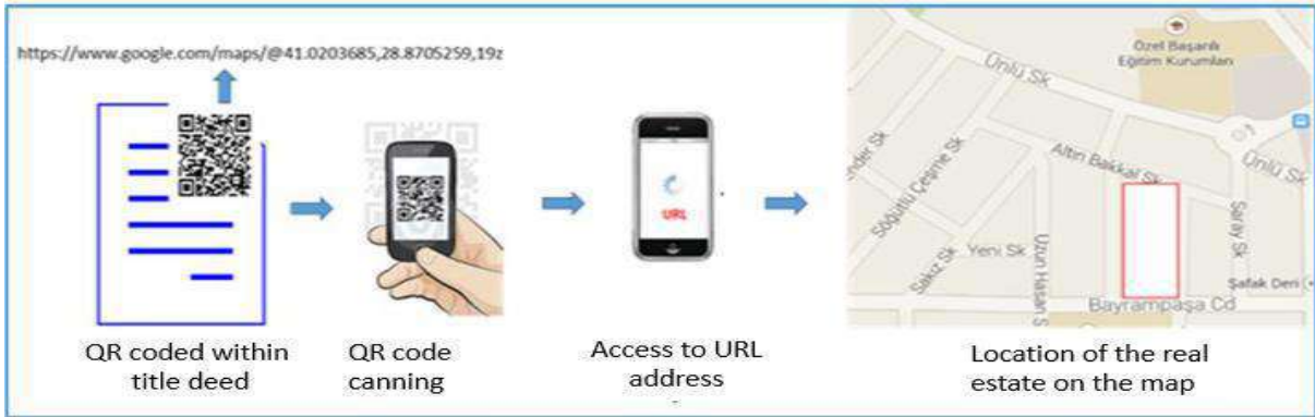
Figure 6: Comparison of the location of the real estate on the map and in the land by using the land registry certificate with the QR code.
