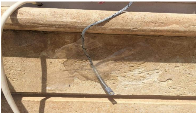
Figure 5. Thermocouples measured ambient and outside temperature
